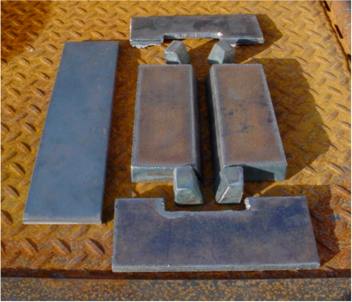
All the pieces to assemble a Single V Groove Weld with Strong Backs.
